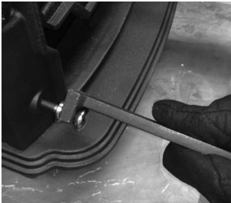
Use the forked end of the Baby Gabriel multi-purpose tool to move the external riddler backwards and forwards to clear ash from the shaker grate as shown
