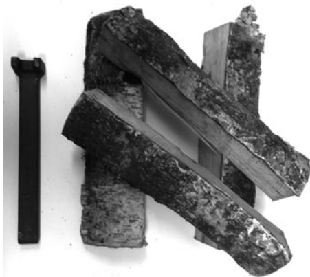
The recommended maximum fuel load: Photo shows a typical loosely stacked fuel load of approximately 1.5kg of fully seasoned wood logs approx 250mm (9") long by 75 – 100mm thick
